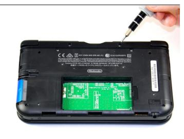
Remove the six 6.2 mm screws using a Phillips #00 screwdriver
