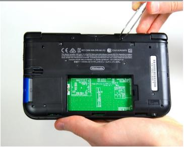
Using tweezers pull out the rubber bumpers that are located at the top of the device on either side of the game cartridge compartment.
