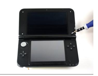
Remove the four 4.3 mm screws located underneath the four rubber pieces with a Phillips #00 screwdriver head.
