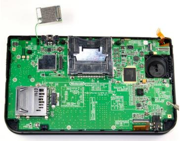
Remove ten 3.0 mm screws that are located around the face of the motherboard.
