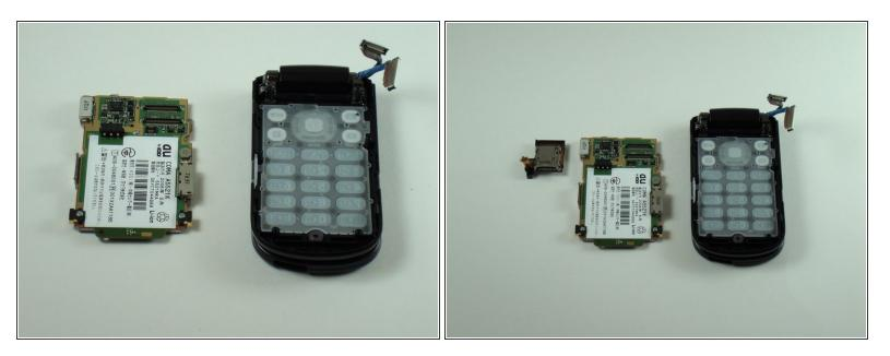
• The logic board should now be completely disconnected from the phone.
