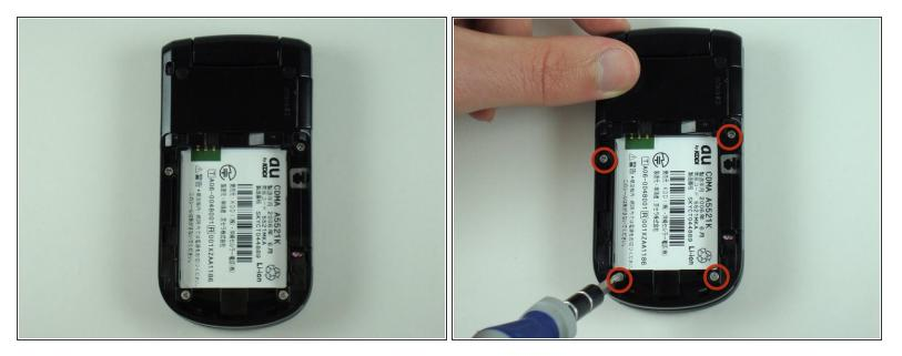
• Remove the four screws with the Y0 screwdriver.
