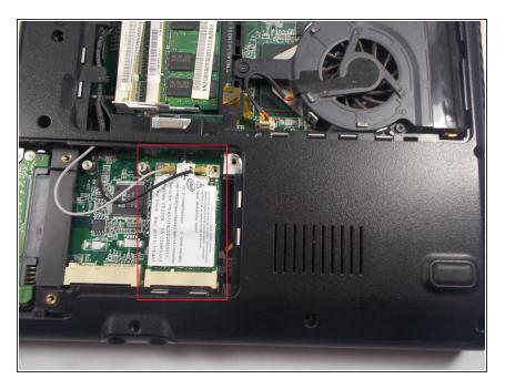
Locate the wireless card on the right side of the now removed panel.
