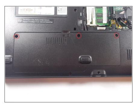
The first thing you need to do is remove the panel concealing the wireless card, by taking out the screws.
