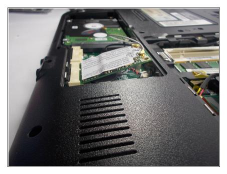
After removing the screws, gently pull upwards on the end of the wireless card until it is angled as shown.
