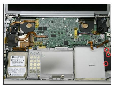
Remove the three 4 mm T8 Torx screws from the PRAM battery board.
