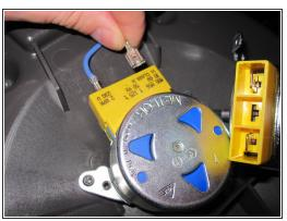
• The motor is now exposed with the bottom cover removed. There are two security screws, the same size as the ones on the outside cover that need removed. There are two wires that need removed from the old motor and inserted into the new motor. The new can be secured in place and tightened with the screws.
