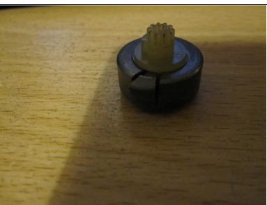
• I took my old motor apart to see why it wouldn't work. I discovered a circular magnet in the bottom, underneath the cogs etc. Upon closer inspection I seen it was cracked and a little pull and it came apart. It made it's way to the bin.
