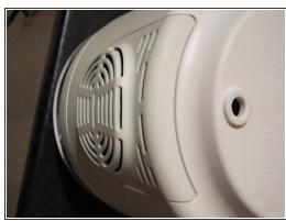
Next remove the three screws and the little fan cover at top end of the unit. I gently prised it off with a butter knife. This allows the bottom plastic cover of the Actifty to come off, from the fan end first, then it slips over the lid release buttons and off.
