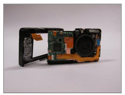
Now that you have removed all of the screws, carefully pull the case apart at the seem. The case will detach from the camera in two pieces.
