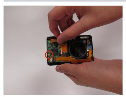
Remove the screw on the far left hand side of the camera.
