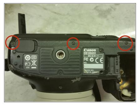
Three screws on the bottom need to be removed next. They can be removed in any order
