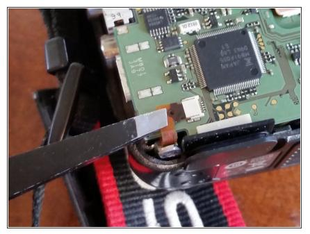
Next to remove is the bottom left corner flex cable. It has no tightening bar, so pull it out with tweezers or with your fingers.
