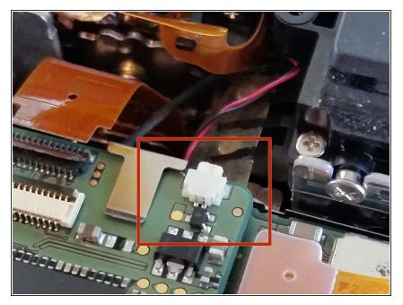
• The red and black power cable can be removed next. It it different than the rest, and can be removed by either using a plastic opening tool or a very small pair of pliers to remove it.
