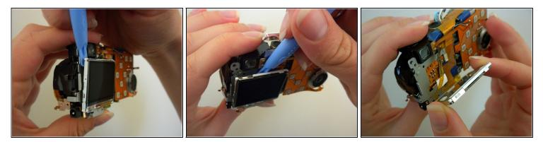
• Pry off the LCD screen from the top using an opening tool.
