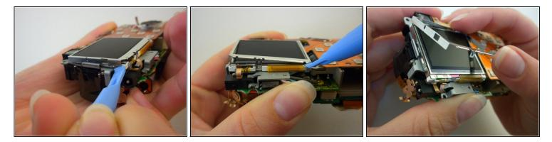
• Remove the metal frame from the LCD screen using an opening tool.
