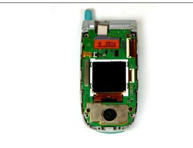
Using a small Phillips screwdriver, gently pry off the LCD screen from the board.
