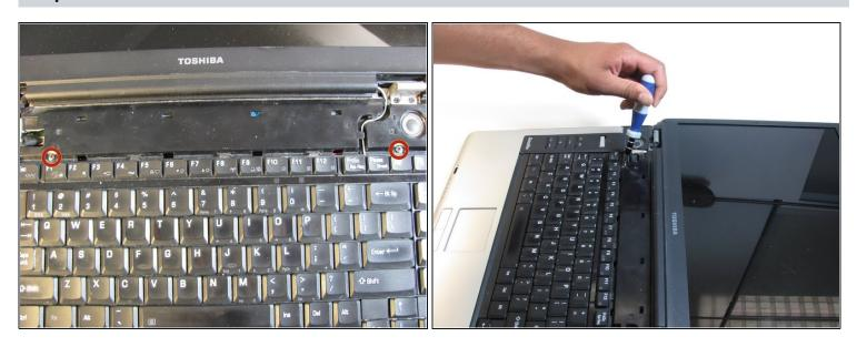
• Unscrew the two 4.5 mm screws holding the keyboard on with the Phillips #1 screwdriver.
