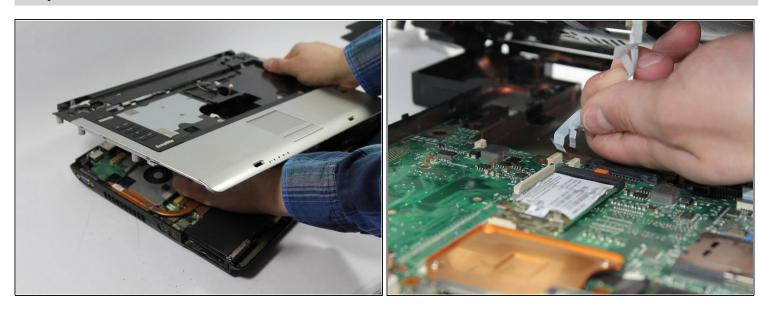
• Lift the top half of the case enough to get your hand beneath it, and then remove the two ribbon cables that connect it to the motherboard.
