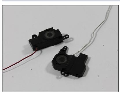
The wires for the speakers are color coded. The red and black wires are for the right speaker, and the black and white wires are for the left speaker.
