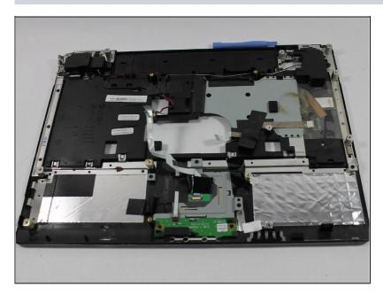
Remove the lower half of the laptop and lay upper half on its top.
