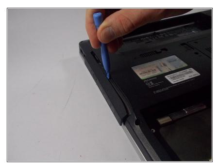
Use any tool with a flat edge in order to pry out the CD-Drive, preferably a plastic opening tool.
