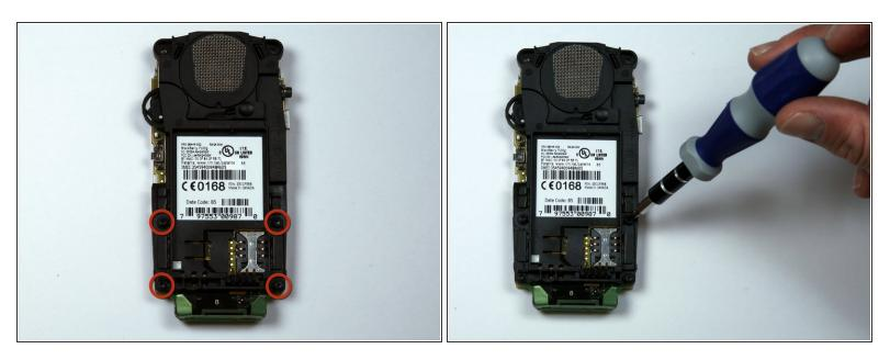
• Remove the four screws holding the battery and speaker housing to the motherboard.
