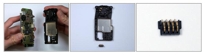
• Once the battery housing is seperated from the motherboard, the battery terminal will slide off the battery housing.
