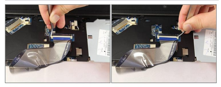
• Using tweezers pull the white tab down on both sides. This will release the blue and black connector.
