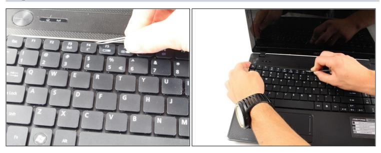
• Using thin <u>tweezers</u> push the tabs in the keyboard in and pull up on the edge of the keyboard.
