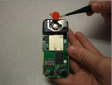
• Remove SOS button from circuit board with tweezers.
