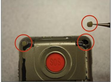
• Remove the four rubber inserts from the screw holes using a pair of tweezers.
