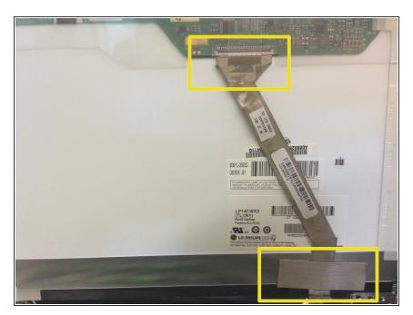
Remove the tape at the spots shown in the picture to detach the screen from the ribbon.
