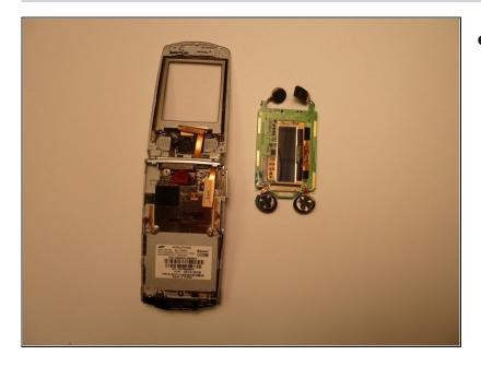
• Completely remove the screen and circuit board unit from the cell phone.
