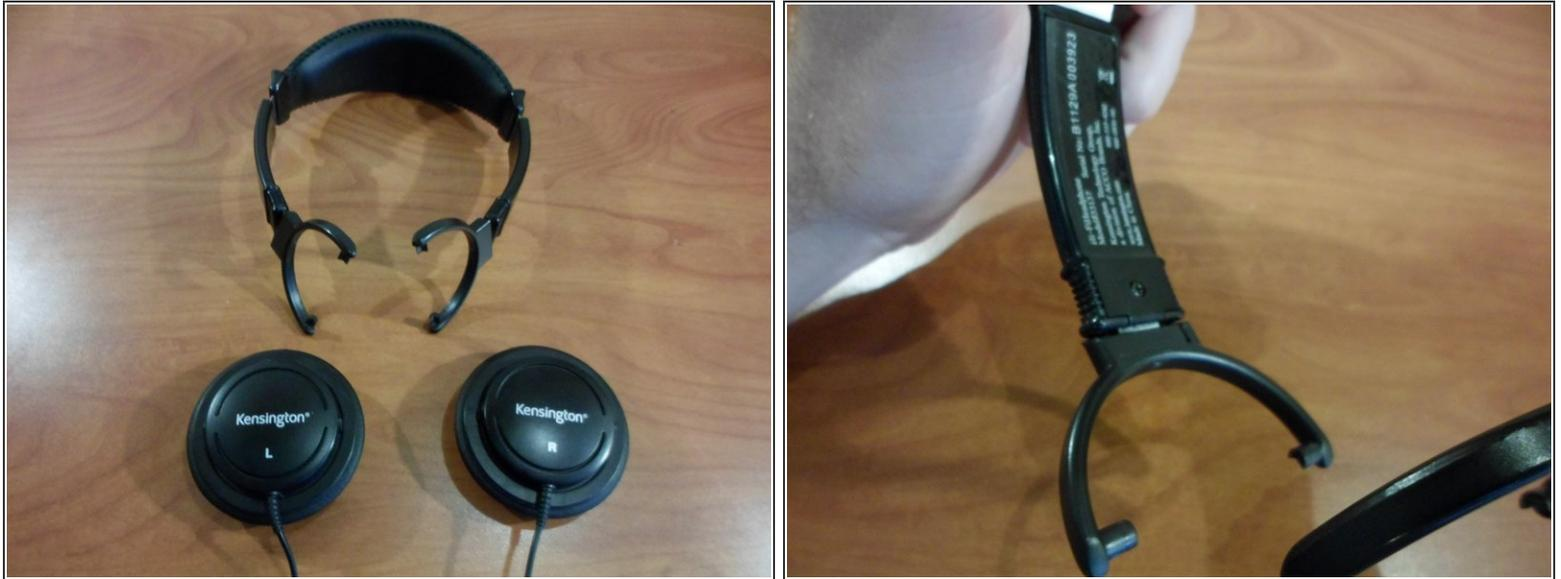
**i** This picture shows the headphones with the speakers detached. Steps 1 and 2 are not necessary to replace the headband covers, however they do make the process easier.
