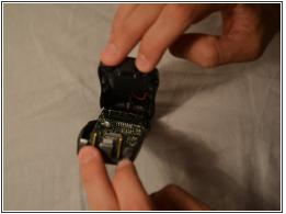
Gently open phone casing along the seam at the bottom of the phone using index and middle fingers of both hands
