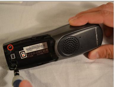
Remove the two 11mm screws inside the battery storage compartment using Phillips #1 screwdriver (located near the very bottom of the phone)
