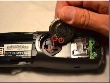
With speaker exposed, remove the speaker by cutting the red and black wires near their contact location To reassemble your device, follow these instructions in reverse order.
