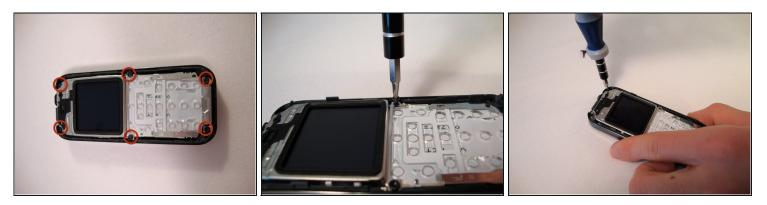
• Remove the six screws found along the frame of the phone with a T6 Torx screwdriver and put them to the side.
