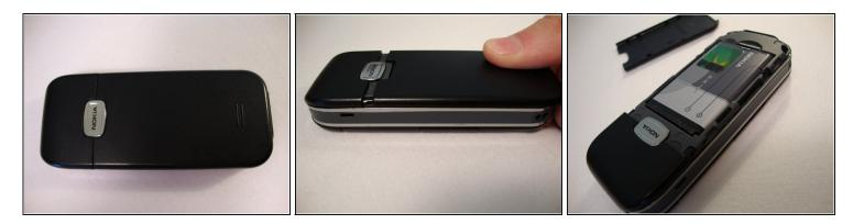
• Press down on the grip on the back of the phone and slide the rear housing down towards the bottom of the phone.
