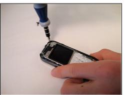
Remove the six screws found along the frame of the phone with a T6 Torx screwdriver and put them to the side.
