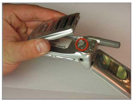
• Pull back on the white release tab and lift up the the entire battery.
