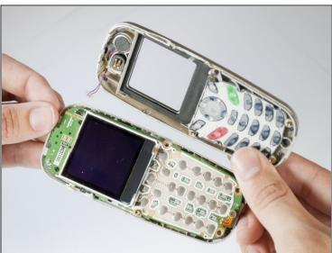
• Using your nails, <u>tweezers</u>, or any precise grabbing tool, pinch the antenna wire connector (clear plastic plug) and pull gently. It should pop out rather easily.
