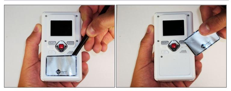
闭 Turn off the device and take the batteries out.
