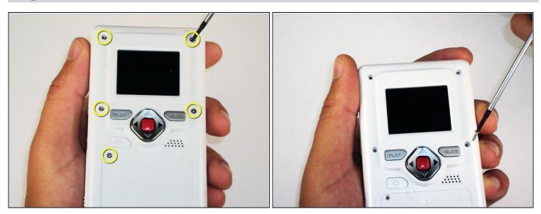
• Remove the 5 10mm screws with the #00 Phillips screwdriver. These connect the back of the outer shell to the front of the outer shell.
