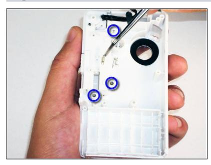
Remove the 3 screws securing USB port cover to the outer case with the #00 Phillips screwdriver.
