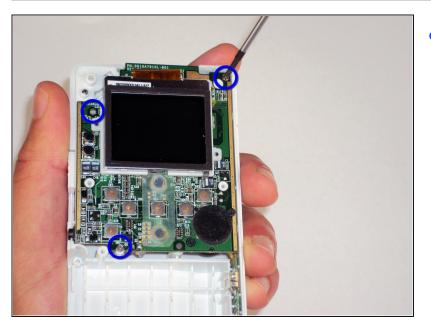
Remove the 3 5mm screws securing the circuit board to the front shell with the #00 Phillips screwdriver.
