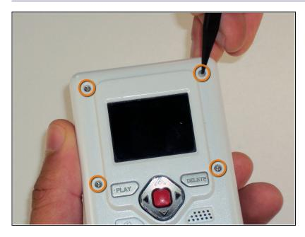
• Remove the 4 gray screw caps with the spudger. These cover the screw heads and protect from dirt or grime.
