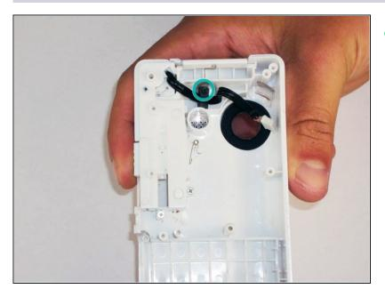
Remove black 3mm screw that secures wire to outer shell with #00 Phillips screwdriver.
