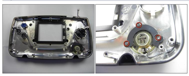
A Removing the plastic holding the speaker to the case may permanently detach the speaker.
