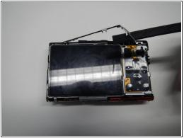
Remove the L shaped bracket around the top and right side of the LCD screen
