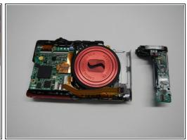
Lift the flash housing up and forward from the top of the camera to carefully remove
