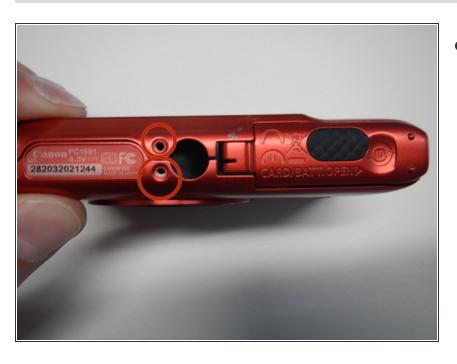
Remove the two screws on the bottom of the camera located near the battery door (Phillips #00 screwdriver) (4.0 mm).
