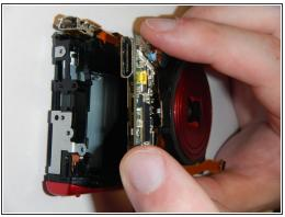
Remove the motherboard from the frame by gently grasping the outside edge and pulling away.
