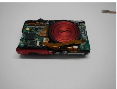
Remove the ribbon wire attached at the bottom right corner of the front of the camera. You do
