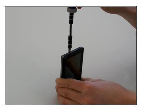
Underneath the piece of plastic you just removed, there is a small screw (Phillips #000, 2.0 mm long). Use a Phillips #000 screwdriver to remove it.
