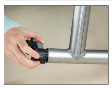
Grasping the hub firmly, slide piece from metal frame. This may require the use of a hammer or other sturdy object, as the hubs are firmly placed in the metal frame.
