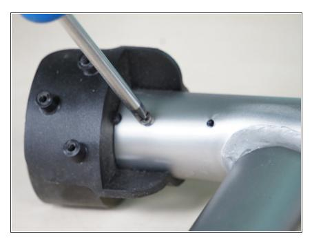
Screw back in the small screws into the metal frame. Make sure the screws are properly aligned with the holes in the hub piece. This will ensure that the piece will stay in place and is secure.
