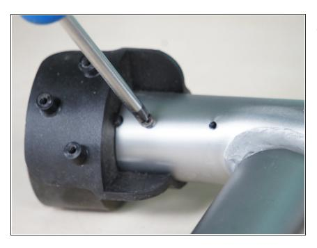
Using the screwdriver, remove the two small screws in the metal part of the frame.
