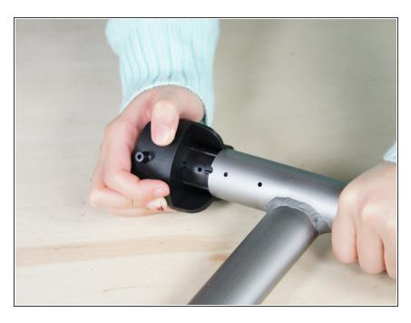
Insert new wheel and hub piece into the metal frame. May once again require a hammer to fit in the new piece snugly.
