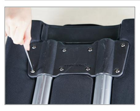
Place metal frame back onto the luggage body. Using the Allen wrench, screw in the 8 bolts back into the backing of the handle frame.
