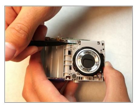
Remove the flash bulb from the camera housing by gently pulling on the wires with a pair of tweezers.
