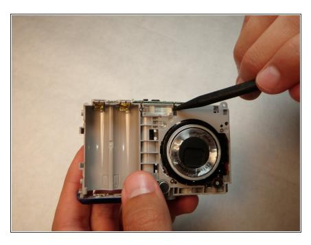
Poke the capacitor out of its housing with the spudger.
