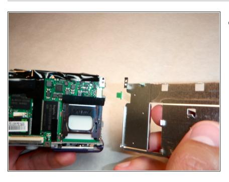
Remove the ribbon cable from its slot by gently pulling the LCD holding plate to the right.
