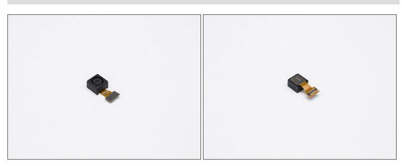
The 5MP camera located on the back of the phone.
