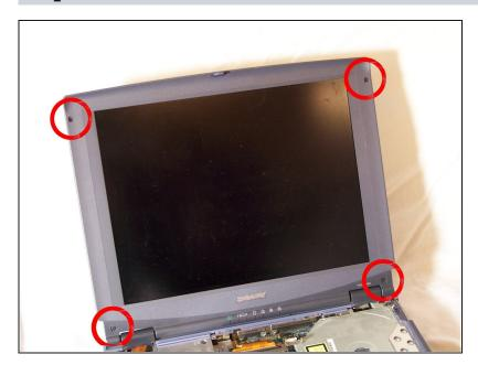
With the screwdriver, unscrew the four screws that attached the front bezel panel with the display assembly, as shown in the image.
