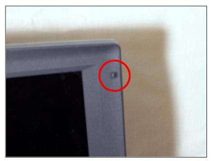
Use <u>tweezers</u> to remove the rubber covers on the four screws at the corners near the display.
