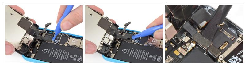
A Make sure the battery is disconnected before you disconnect or reconnect the cables in this step.
