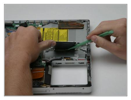
Lift the modem up from the left side and use a spudger to disconnect the cable attached to the bottom.
