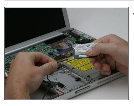
Disconnect the modem cable from the modem.
