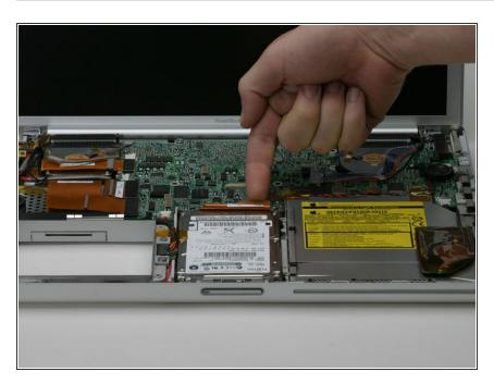
Disconnect the large orange hard drive cable from the logic board, removing tape as necessary.
