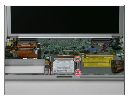
Remove the two 6 mm long silver Phillips screws from the metal bracket to the right of the hard drive, removing tape as necessary.
