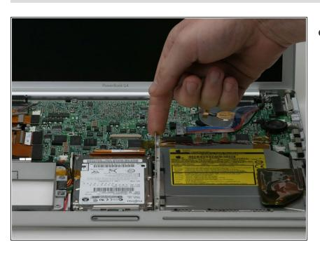
Use a spudger to lift the metal bracket out of the computer.
