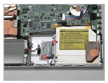
Remove the two black Phillips screws from the modem board.
