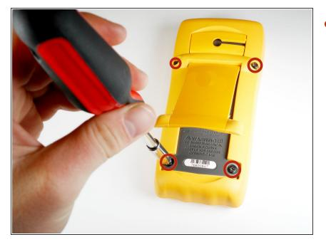
Use your Phillips #2 Screwdriver to remove the four black 21 mm Phillips #2 screws.
