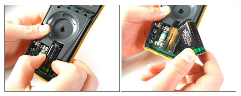
Mhen doing this next step, make sure to remove the battery slowly, so you don't damage the wires connecting the battery to the device.
