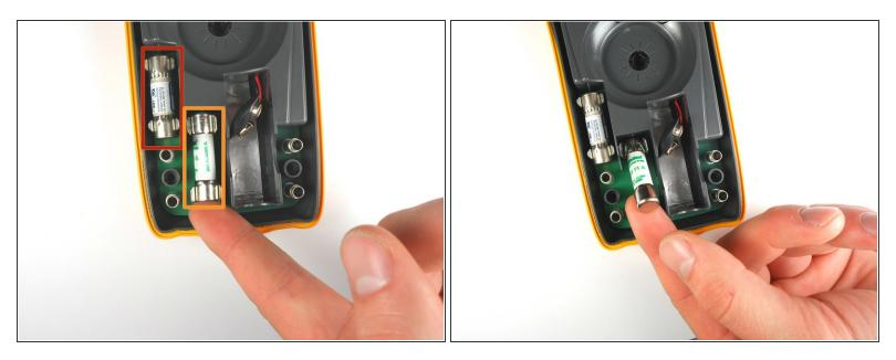
Replace a fuse only with a fuse identical in type, voltage rating, and current rating as specified by the back panel fuse rating label or the <u>Fluke 77 Series III Service Manual</u>. Inserting the wrong replacement fuse could create a fire hazard.
