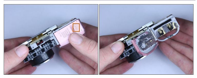
• Open the battery door by pulling in direction of arrow
