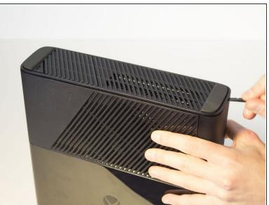
Slide the spudger along the crevice to separate the grated face and the top body.
