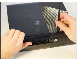
Beginning on the left side without the grate, run the spudger along the crevice until you've reached the grated part, while holding the part that's being separated as you go.
