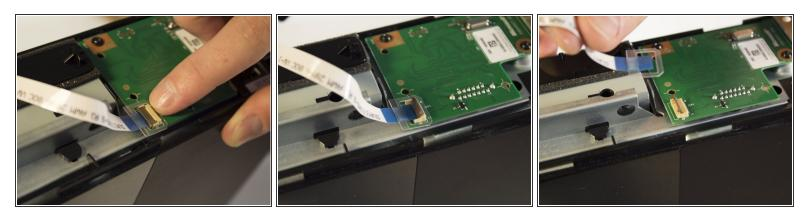
• Find the brown section where the ribbon cable enters the green board. Flip the brown part up and pull out the plastic tab at the end of the ribbon.
