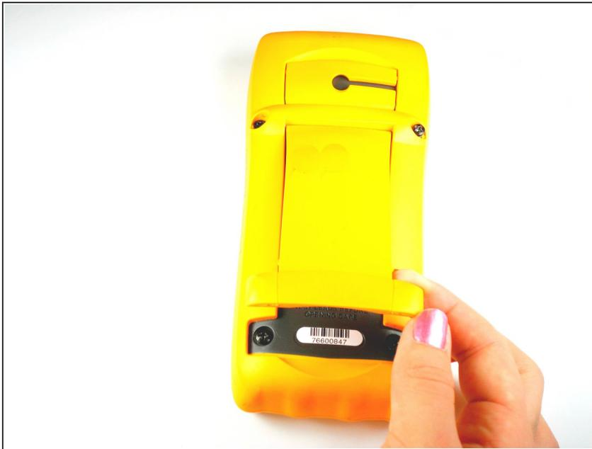
**⚠** Be sure any test leads are out and the multimeter is off before opening the device.
