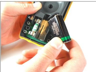
Mhen doing this next step, make sure to remove the battery slowly, so you don't damage the wires connecting the battery to the device.
