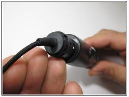
• To check the cord further by unscrewing the bottom piece of the microphone from the top. Rotate clockwise to unscrew the bottom and examine.
