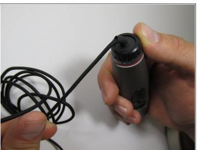
Inspect the cord for splits, breaks, or loose wires. Check the cord from one end to the other, making sure the cord is attached to the microphone.
