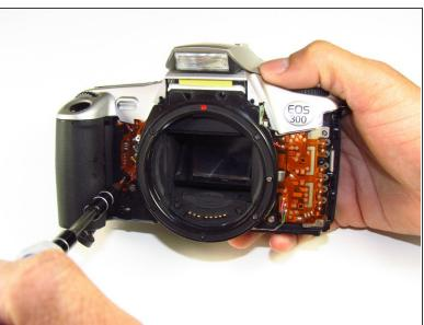
Remove two black 4.8mm Phillips #1 screws on the front of the camera.
