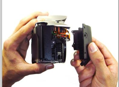
Pry open the side grip using a spudger.
