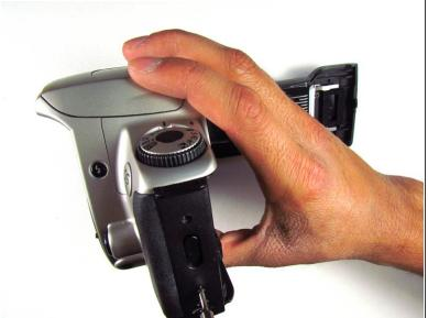
Remove the two black 4.5mm screws above and below the latch.
