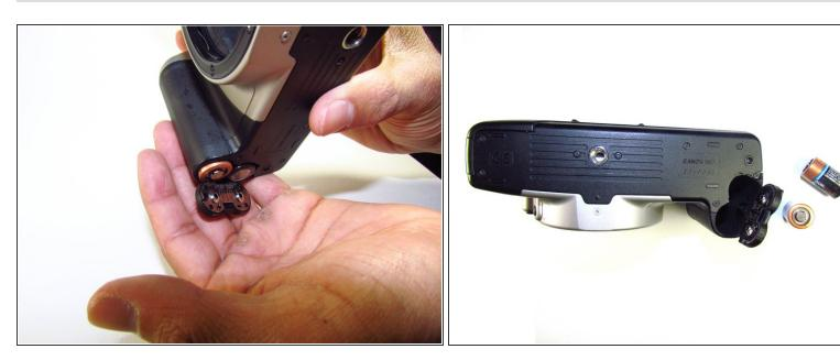
Remove the batteries from the camera by sliding them out into your palm.
