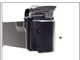
Remove the remote control socket cover.
