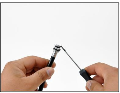
Replace the 3 O-rings on the ABS hose. Use a small flathead screwdriver to help pry the old O-rings off and stretch the new O-rings on.
