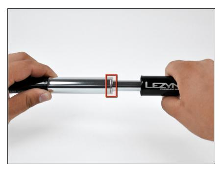
Pull the pump plunger up until the silver cap is exposed.
