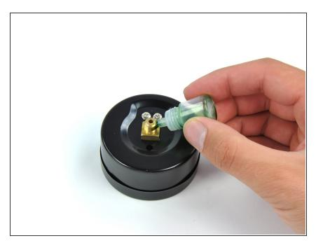
Apply medium-strength Loctite (green, 290) to the threads of the new gauge.
