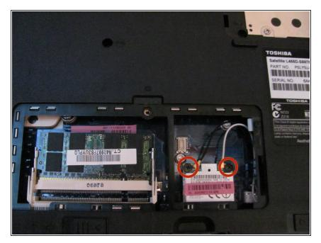
Remove the two Phillips #1 6mm screws from the wifi card using a Phillips #1 screwdriver.
