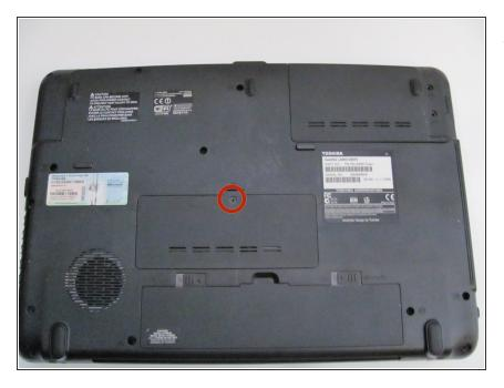
Unscrew the Phillips #1 4mm screw from the middle panel using a Phillips #1 screwdriver.
