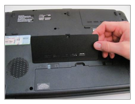
Remove the middle panel by lifting up and out.
