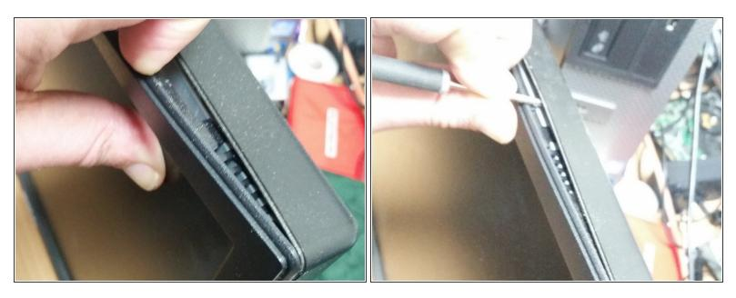
Best to do this with the screen facing down so you don't rip out the ribbon cable that attaches to the buttons on the front of the screen, start in the middle of the bezel to get purchase then slip a screwdriver underneath to gently prize up the bezel working along until its released, the edges are stubborn but do release with patience
