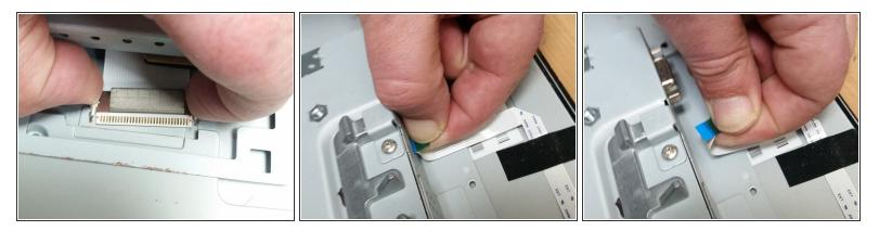
• The small ribbon cable is easy to remove gently pull (see picture), the larger ribbon cable can be stubborn I tend to use two screwdrivers one to push in the release catch and the other flat bladed one to gently wiggle it out, same procedure for the other side, if you get image corruption after the repair this is the cable that is the culprit
