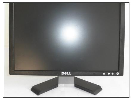
1. remove plinth from monitor by pressing the button on the back of the screen
