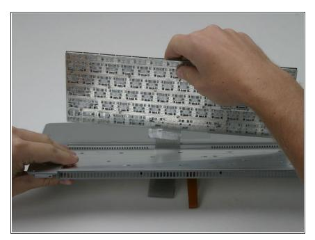
Pull the freed keyboard directly up, minding the cable as it slides through the slot in the casing (watch out for the adhesive on the underside of the case).
