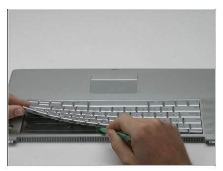
Lay the casing flat so that the keyboard faces up and and slowly pry the keyboard up, beginning at the back edge along the 'F' keys, and moving toward the space bar.
