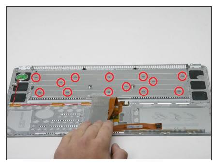
Remove the 13 identical Phillips screws attaching the keyboard to the casing.
