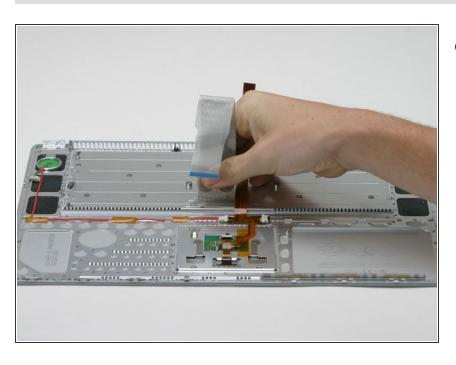
Peel back the grey keyboard ribbon from the metal casing.
