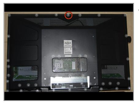
Step 1 - Remove all 42 screws from back cover. Remove top center screw last, it will help to hold the panel in place during removal of other screws.
