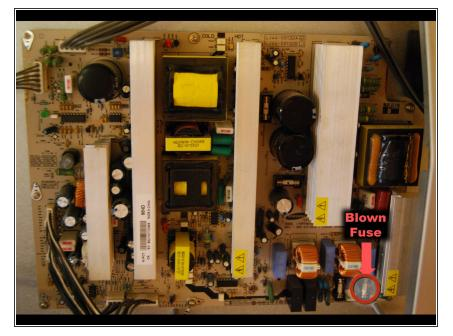
That's the one that I found faulty. Just Remove it with a pair of needlenose pliers and replace with a new one (ft8ah250vp).
