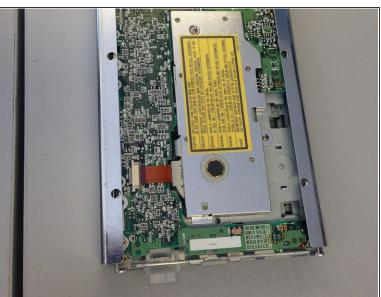
Slide metal panel out of the metal casing.
