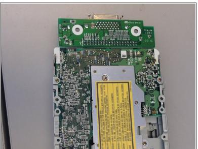
Slide disk drive out of metal casing.
