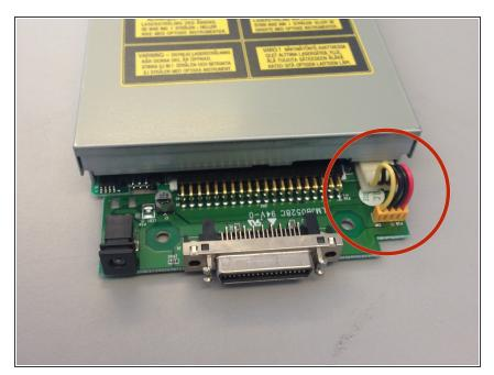
Flip the disk drive over so the the plug on the daughter board is visible.
