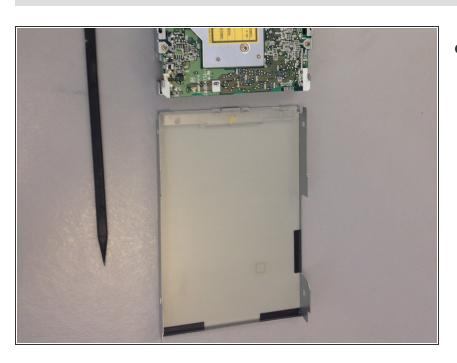
lift the disk drive completely out of the metal casing and set it aside.
