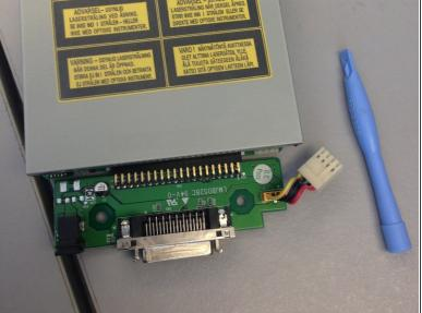
Using an iPod opener put pressure on the white plug and pull backwards until the daughter board unplugs from the main unit.
