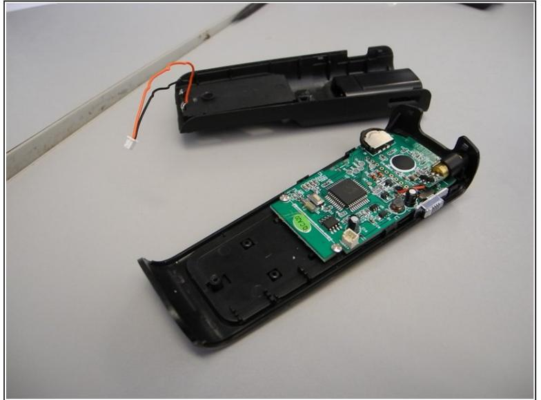
**⚠** There is a wire connector linking the front and the back of the device.
