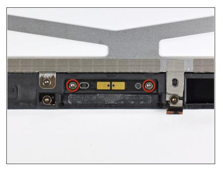
Remove the two T5 Torx screws securing the home button switch board to the display frame.
