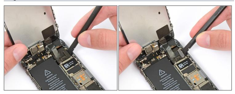
• Use a spudger or a fingernail to disconnect the front-facing camera and sensor cable.
